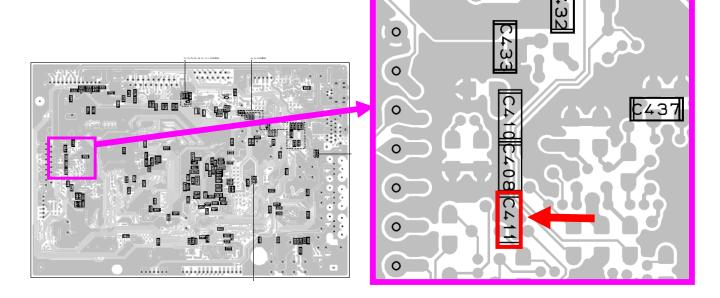
**SERVICING:** Regardless of the symptom, check and remove C411 from all units sent in for service.
