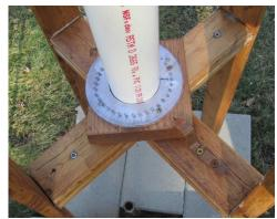
(Pic above) The base of the outer pipe, with a compass rose attached, is supported on a wooden plate which is affixed to a 3 inch 'Lazy Susan'. This assembly permits the antenna to be easily rotated. (The 'Lazy Suzan' is not is view in this picture but can be seen in the version at my TN QTH pictured next.)
