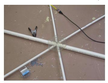
(Pic left) On loops requiring spoke support to maintain structural integrity, 1/4 inch thick Plexiglas gusset plates are used to lock the spokes to the PVC antenna pole. A short section of a 1 inch diameter wooden dowel is positioned inside the antenna pole directly beneath the gusset plate to strengthen the screw hold.
