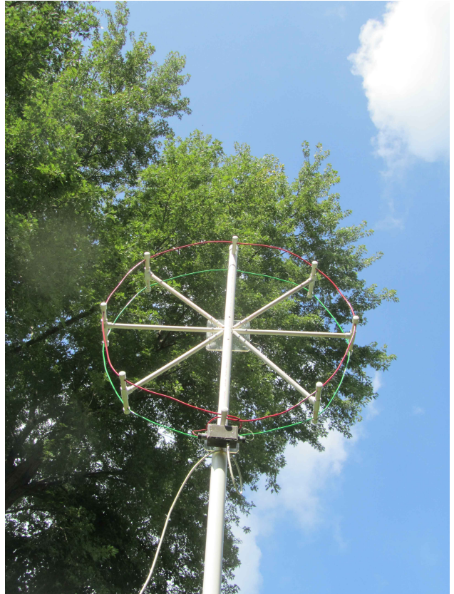
(Pic above) Two-turn Parallel-connected loop at the NJ QTH ... distinguished by red/green loop wire. A picture of the TN version ... distinguished by black/white loop wire ... is shown on the next page.
