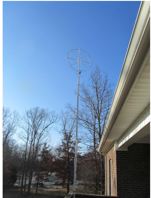
(Pic Right) LZ1AQ Two-turn Parallel-connected Loop at 30 feet at the Middle Tennessee secondary QTH.
