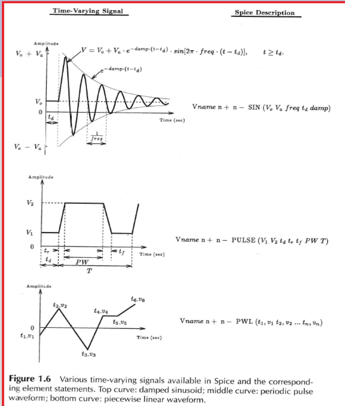
**Figure 1.6** Various time-varying signals available in Spice and the corresponding element statements. Top curve: damped sinusoid; middle curve: periodic pulse waveform; bottom curve: piecewise linear waveform.
