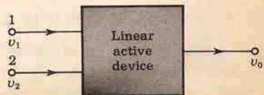
Fig. 15-5 The output is a linear function of v_1 and v_2 for an ideal differential amplifier; v_o = A_d(v_1 - v_2) .
