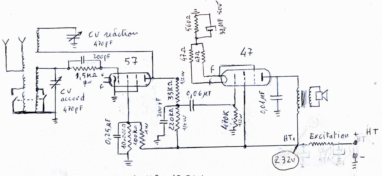
Tension aux bornes transfo HP 17,50V
