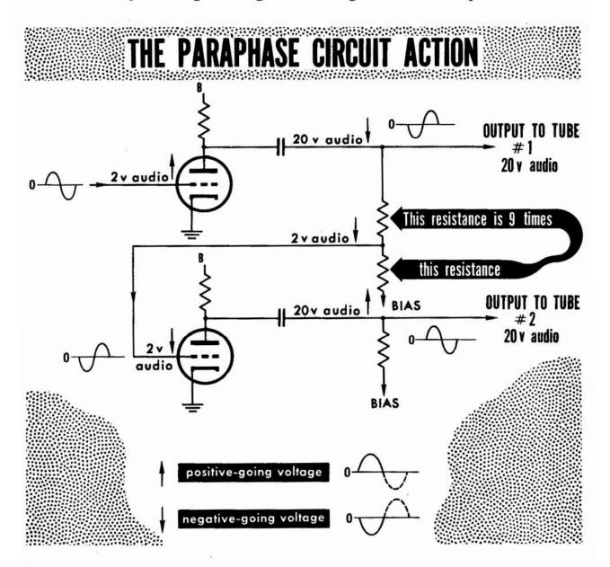
A positive fluctuation of 2 volts at the grid of the first paraphase tube produces a negative fluctuation at its plate of, say, 20 volts, which appears at the grid of one of the output tubes. This 20-volt fluctuation is also divided to provide a negative fluctuation of 2 volts for the grid of the second paraphase tube and becomes a positive fluctuation of 20 volts at the plate, providing positive fluctuation for the grid of the second output tube.
