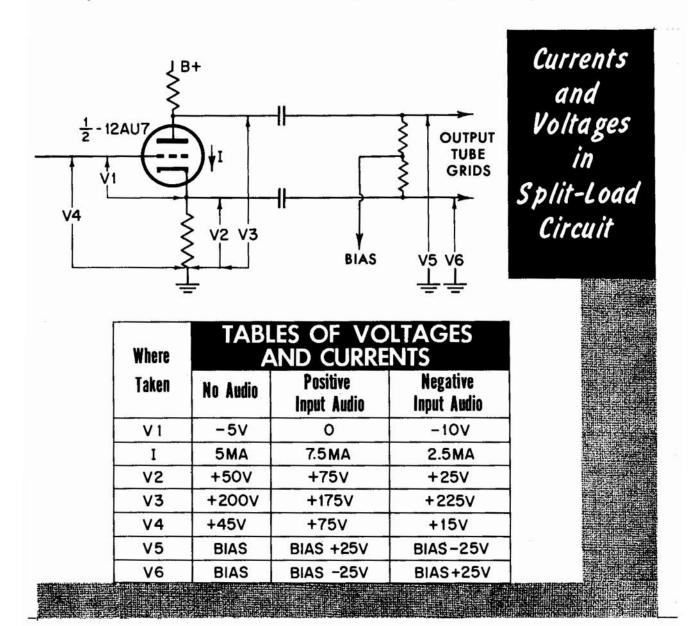
this, the grid-to-ground voltage itself must go 25 + 5, or 30 volts more positive to produce this swing. We therefore require a 60-volt peak-to-peak audio fluctuation from grid to ground to produce a 50-volt peak-to-peak fluctuation at plate and cathode respectively.
