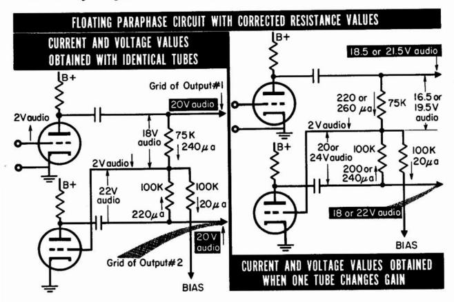
The unbalance between output tube grids can be corrected by using a smaller resistance value from the first output tube, so that 240 microamps only drop 18 volts. This requires a resistor of 18/0.00024 = 75,000 ohms, in place of 100,000 ohms.
