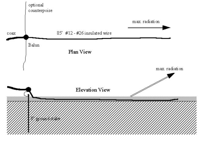
These antennas are largely resistive, with values ranging from 150 to 500 ohms or so on average ground. They have been used successfully on the average soils northwest of Washington, DC, on the sandy soils of the Cape Canaveral, Florida area, in the rocky, shale soils of the mountains in Somerset county, PA, and on river bottomland of Allegheny County, PA. One was used with great success by K3MT/VP9 in Southampton, Bermuda - the object of nightly pileups on 30 m CW for four nights.
