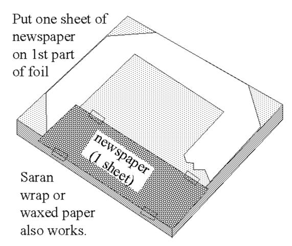
Leave the fifth flap of foil loose, so it can be lifted up when necessary. Cut off excess foil so it does not short circuit against the foil beneath the newspaper.
