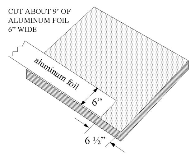
Fold the foil over itself as shown. Use tabs of scotch tape to hold the foil in place. Continue taping it down on three, and part of the fourth, side:
