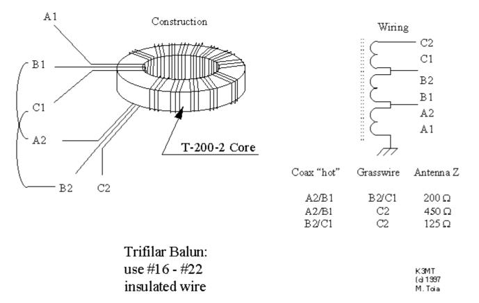
Typically I pull the insulation off of some indoor telephone wiring cable. Four insulated #22 copper wires are inside: discard one of these and use the remaining three. Wind about 16 turns on the core, without allowing the wire to twist (keep the three conductors parallel at all times.)
